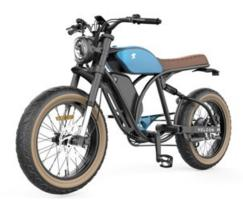
We began taking pre-orders for the 2023 Volcon Brat E-Bike in September 2022 and expect shipments to customers to begin in the fourth quarter of 2022. Similar to the lineup of Volcon motorcycles, the Brat will have a low seat height, large tires, hydraulic front and rear disc brakes and is expected to be a Class 2 E-Bike capable of achieving 20 mph maximum speed from throttle assistance. The Volcon app will also work with the Brat.
